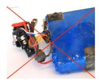
Cables with open ports or bare parts have to be cut so that no bare stranded wires are visible. Cut the wire as close as possible to the battery.
